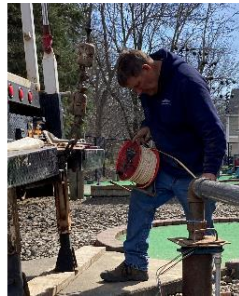
Image 5: Step-Down Pump Test
