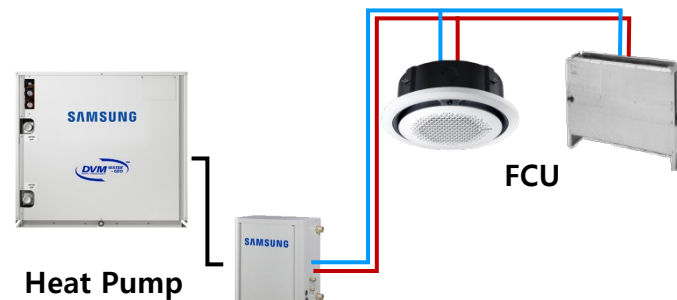
Fan Coil Unit Heating/Cooling
